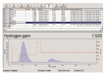
The advanced furnace control of the RHEN602 software facilitates the analysis of surface and bulk hydrogen in aluminium
