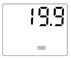
If you want to measure and compare more than one sample, press the key. The last measured value is stored and appears in the lower display line. The upper display line continues to show the current measured value. If the print function is switched on, the value can also be output on the RS232 interface by pressing the key
