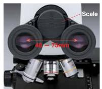
adjustment and diopter setting. High eyepoint design eyepieces with F.N. 20 can be used comfortably without removing eyeglasses.
