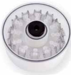
**4446** - DOUBLE sample disposable holder complete with white filter card (up to 1ml samples). Cell deposition area 6mm in diameter.
