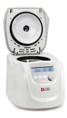
DLAB hematocrit centrifuge with AC24P hematocrit rotor is used for determination of volume fractions of erythrocytes in blood for diagnostic purposes and doping tests. Also it is used to derive plasma for the photometric determination of the bilirubin content of the blood of neonates.
