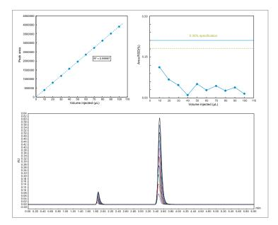
Injection precision for the 100  $\mu$ L syringe: Analysis of a wide dynamic injection range showing chromatographic overlays, injection linearity, at >0.2%.
