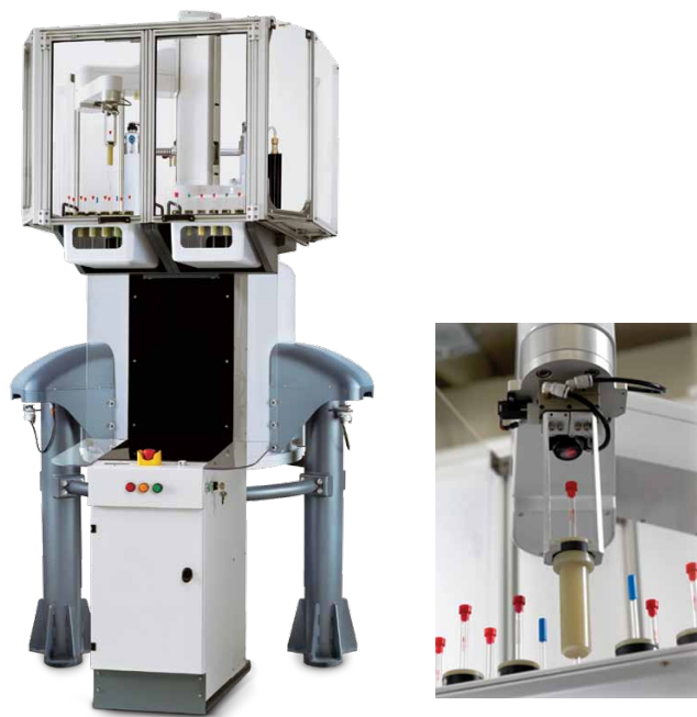
7620-AS autosampler (left) with close-up of robot handling sample (right).
