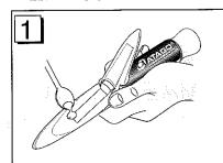
Put one or two drops of sample on the prism.
