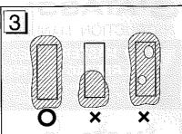
The sample must spread evenly over the prism surface. Air bubbles should be eliminated.
