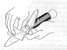
※ After each measurement, wipe the sample off the prism, daylight plate, and around the prism area with a soft most tiesus.
