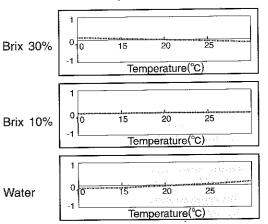
Note: The temperature compensation coefficient set for the MASTER- $\alpha$  corresponds to a Brix of 10% to15% When water is measured the boundary line may deviate slightly from the 0% line, however the accuracy is within specification.
