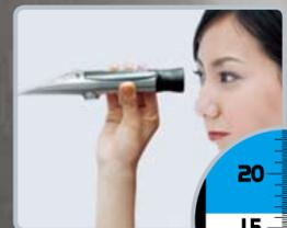
3 Read the measurement value where the boundary line intersects the scale.
