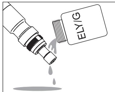
Rinse the sensor head with electrolyte solution.
