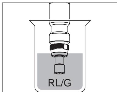
Immerse the sensor head including the counter electrode in RL/G cleaning solution.
