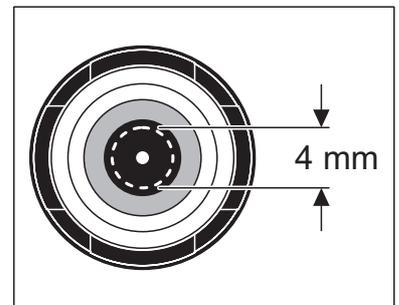
Check the filling: Inspect the face surface. No air bubbles may be present within the dashed circle (approx. the black area). Air bubbles outside this area do not interfere.
