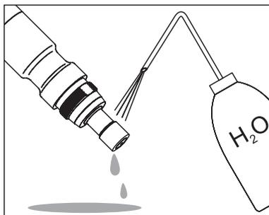
Rinse the sensor head with deionized water.
