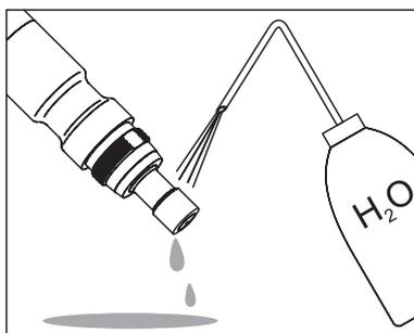
Rinse the sensor head with deionized water.
