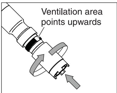
Hold the sensor inclined and screw on the membrane head fingertight using a paper towel. Excess electrolyte solution is forced out of the ventilation area.
