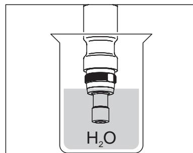
Water the counter electrode in deionized water for at least 10 minutes.
