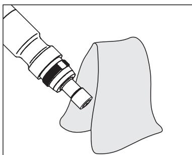
Wipe the counter electrode with a lint-free paper towel and carefully remove any loose white deposits.
