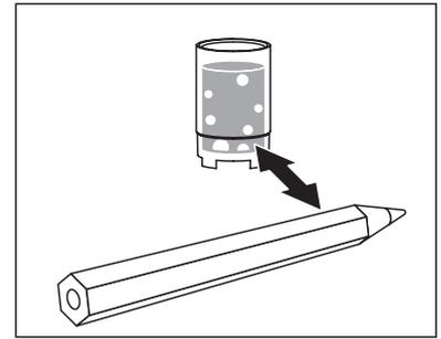
Remove any air bubbles by carefully tapping the membrane head. Additionally, you can prevent air bubbles by throwing the first fill away and refilling the membrane head.
