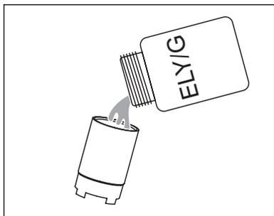
Fill a new membrane cap with ELY/G electrolyte solution.
