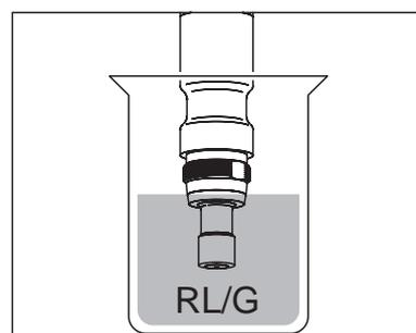
Immerse the sensor head including the counter electrode in RL/G cleaning solution. Allow to react for 1 to 3 minutes.
