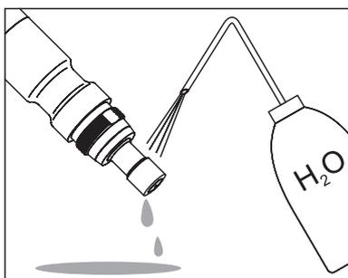
Rinse the sensor head with deionized water.
