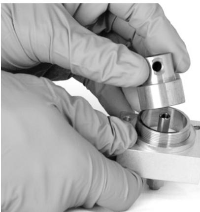
**9** If only replacing the FID castle, skip to step 15 for reassembly.
