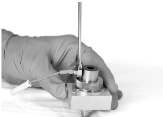
**17** Lower the collector assembly into the housing.
