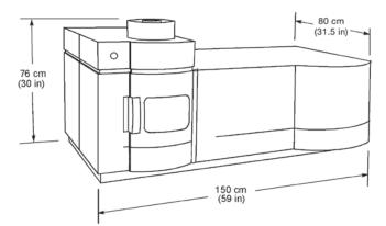
Figure 3. Spectrometer dimensions of the Optima 7300 V and 8300 ICP-OES.
