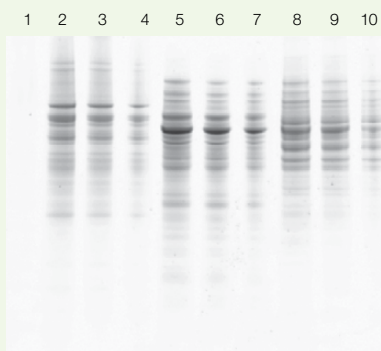
Fig. 7. High transfer efficiency of Mini-PROTEAN TGX precast gels. Mini-PROTEAN TGX or NuPAGE Bis-Tris gels were loaded as follows: lane 1, 5 \mu l Precision Plus Protein unstained standards; lane 2, 15 \mu g mouse liver; lane 3, 10 \mu g mouse liver; lane 4, 5 \mu g mouse liver; lane 5, 15 \mu g E. coli ; lane 6, 10 \mu g E. coli ; lane 7, 5 \mu g E. coli ; lane 8, 15 \mu g mouse brain; lane 9, 10 \mu g mouse brain; lane 10, 5 \mu g mouse brain. Gels were run using Tris/glycine/SDS buffer for TGX gels or MOPS buffer for NuPAGE gels. The proteins from the gel were then transferred onto nitrocellulose membrane in a Mini-PROTEAN Tetra cell using the Mini Trans-Blot module at 150 V (constant voltage) for 15 min with pre-chilled Towbin buffer. Protein transfer was evaluated by staining the membrane with SYPRO Ruby blot stain and imaging on the PharosFX™ imager (A). Proteins remaining in the gel following transfer were visualized by staining with SYPRO Ruby gel stain and imaging with the PharosFX imager (B).
