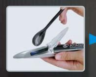
1 Apply 1-2 drops onto the prism.
