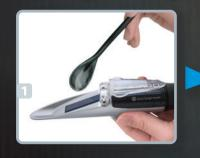
Apply 1-2 drops onto the prism.
