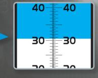
3 Read the measurement value where the boundary line intersects the scale.
