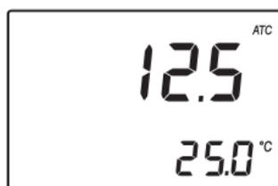
**Note:** The "ATC" tag blinks and automatic temperature compensation is disabled if the temperature exceeds the 0-40 °C / 32-104 °F range.
