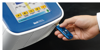
Figure 6. USB functionality on the Veriti® Thermal Cycler.
