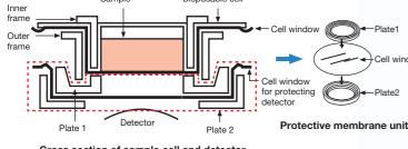
Cross section of sample cell and detector
