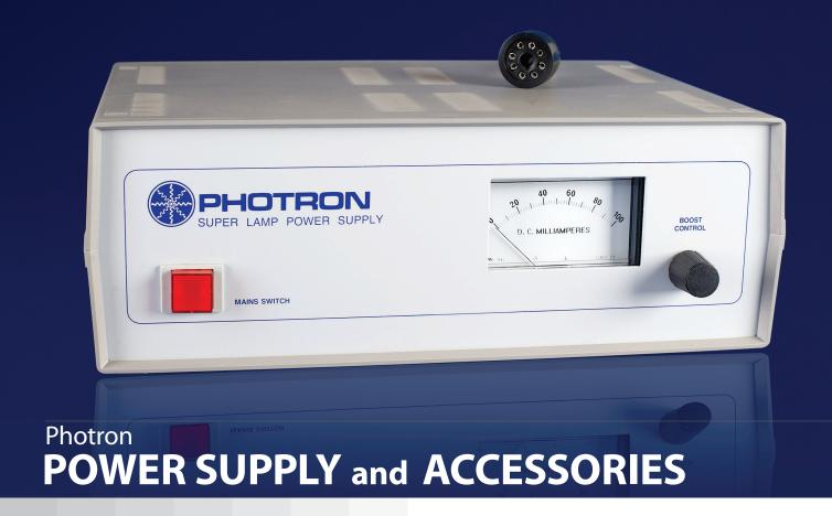
The Photron Super lamp power supply adds a boost discharge for use with Super lamps, the lamp uses existing spectrophotometer lamp current, the power supply adds a boost discharge to increase excitation of atoms sputtered by the instrument lamp supply. This boost current is linked by circuitry inside the power supply and the boost discharge is transmitted at the same rate as the instrument.
