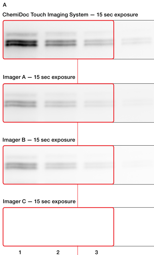
Fig. 3. Comparison between the ChemiDoc Touch Imaging System and other digital imagers. A , Western blot analysis for p44/42 MAPK (Erk1/2) expression was conducted using 2X serial dilutions (starting at 10 µg protein) of Jurkat cell lysate. The membranes were imaged on either the ChemiDoc Touch Imaging System or digital imagers from other vendors for a 15 sec exposure. As shown, the ChemiDoc Touch Imaging System is able to produce images with better definition and differentiation between closely spaced bands. B , The graph demonstrates the ability of the ChemiDoc Touch Imaging System to detect the same faint bands with greater intensity.
