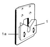
Figure 5. Solid sample slide showing V-holder (1) and spacer (1a)
