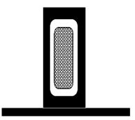
Figure 4. Single cell holder aperture. The thatched area in the middle shows the beam image
