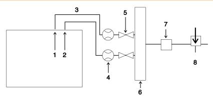
Figure 11. The position of flowmeters when purging with nitrogen
