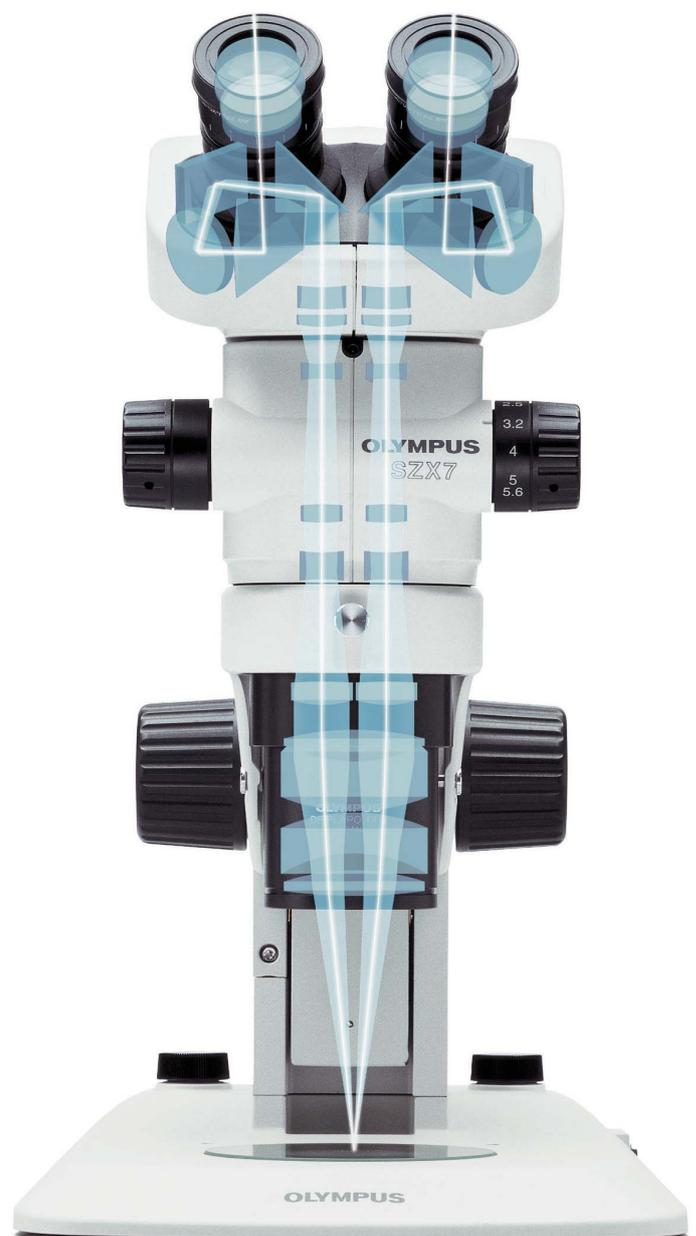
*Galilean optics feature two (right/left) independent and parallel zoom optical paths to produce the focal point with one objective. The system enables high optical performance as well as functional modularity.*
