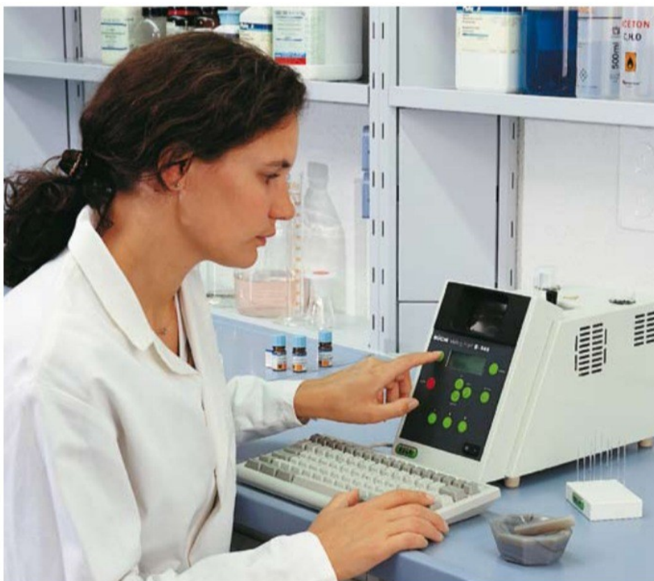
The large magnifying glass makes possible fatigue-free observation of the samples.
