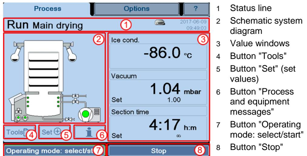
Fig. 19: Overview of the main window "Process"
