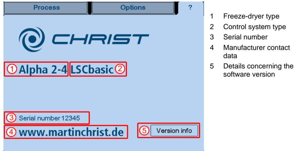
Fig. 48: Freeze-dryer system information (example)
