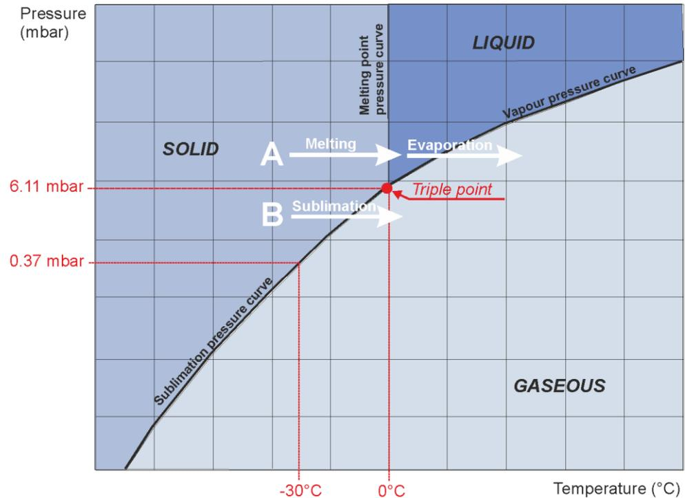
Fig. 7: Vapour pressure curve for ice and water
