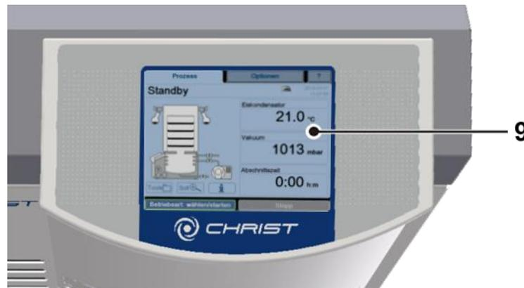
Fig. 60: User interface with touchpanel
