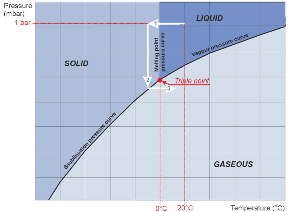
Fig. 8: Freeze-drying phases
