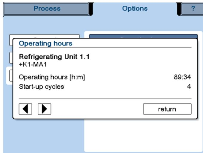
Fig. 44: Dialogue box "Operating hours" (here: refrigeration unit 1.1)
