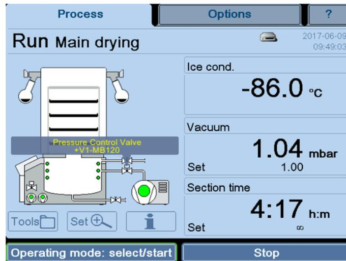
Fig. 20: Schematic system diagram with the name and reference designation of the component
