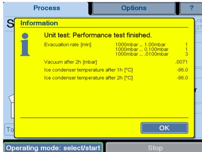
Fig. 29: Results of the performance tests
