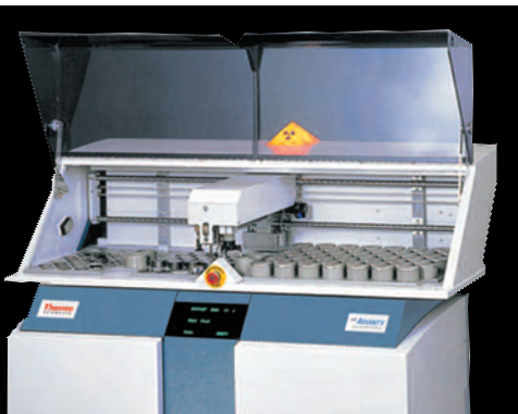
The large sample changer fits directly on top of the instrument
